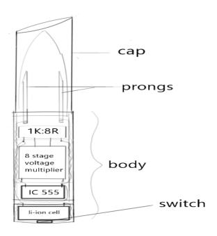
This circuit produces a very high voltage and care must be used to prevent getting a nasty shock. The transformer can produce over 1,000v and the 8-stage multiplier can produce up to 20,000v
